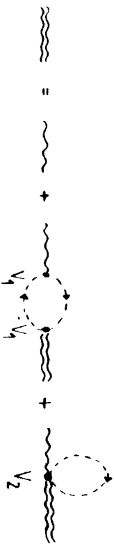
Fig. 1. Diagrammatic representation of the phonon propagator drawn as a double wavy line. The bare phonon propagator is represented by a single wavy line. The phonons interact with the rare earth ions via the linear interaction V_1 and the second-order interaction V_2 as contained in
